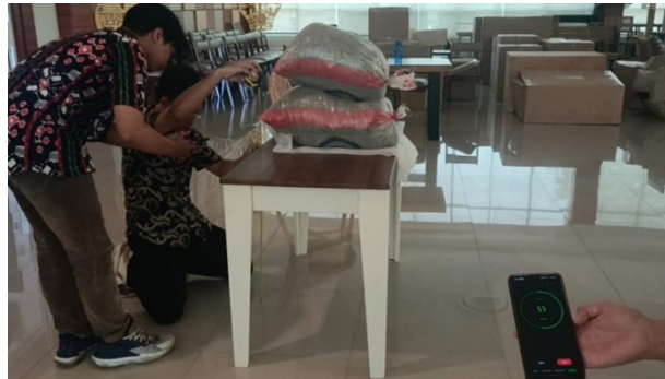
Gambar 10. Proses Uji Beban Figure 10. Load Testing Process Sumber: Dokumentasi Pribadi, 2023
